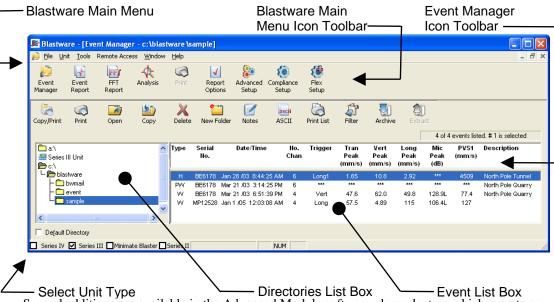
Select Unit Type \_\_\_\_\_ Directories List Box \_\_\_\_\_ Event List Box Several additions are available in the Advanced Module software, dependent on which reports or features you have accessed. In the Blastware Main Menu Icon Toolbar, there is the addition of the Analysis and Advanced Setup icons. Also, within the Blastware Main Menu, there are additional menu selections under Tools, and the Process menu, which is only available when you are performing an analysis of an event.
