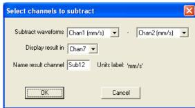
Select the two waveforms to subtract in the first two drop–down menus. Choose where to display the newly created waveform in the Display result in drop–down menu. By default, Blastware creates a new waveform window to display the waveform. If you wish to choose another window, click on the Display result in drop–down menu.
