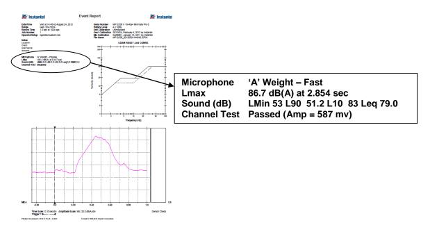
Opening a Waveform or Histogram event that was recorded in Advance mode will produce an event report that shows the Peak Sound Pressure Level (PSPL), when the peak occurred relative to the trigger time, the range the event was recorded in and the measurement units.
