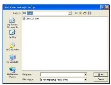
Select a setup file. All setup files have an .evm extension and appear in Blastware's dbase subdirectory. Click **OK** to load the file. To exit without loading a setup file, click **Cancel**.
