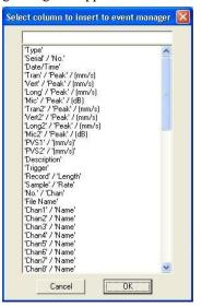
This dialog box lists all the columns that can be used in the Event List. Please see the following table for a description of each column. To insert a column, select a name then click the **OK** button. Click **Cancel** to close the dialog box without inserting a column.
