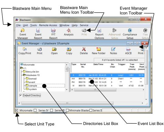
The Blastware Main Menu contains several commands to program the unit. After you have changed the setups, Blastware can transfer the changes to the monitor. In order for Blastware to complete this successfully, a unit must be connected to the computer using the communication cable that was provided with it. Before you enter this menu and attempt to change the setups, connect a monitor to your computer
