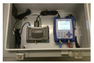
**Mounting Panel Installed in the Enclosure**
