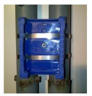
**Micromate Attached with Metal Straps**
