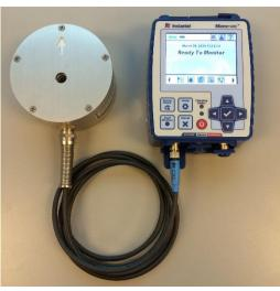
Geophone Connected to the Micromate
