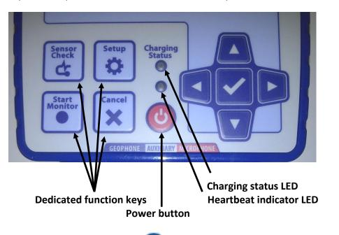
Navigation arrow keys and central check mark key
