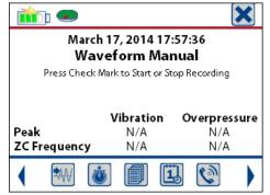
Sample Display for Manual Waveform Monitoring
