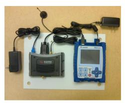
**Micromate Connected to Modem**
