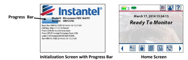
**NOTE:** If the battery indicator (located in the top left corner of the display screen) does not indicate a full charge, which is designated by four green bars, then the Micromate should be connected to an AC power source with the supplied charger. Refer to section <u>12.1 Charging the Battery</u> for additional information.
