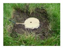
Geophone - Spikes Installed Geophone - Spiked in Ground Geophone - Partially Buried
