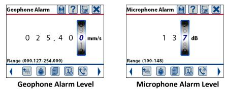
Edit the alarm levels using the keypad of use a finger swipe on the spinner wheel. Once the level has been set press the save icon to save the changes.
