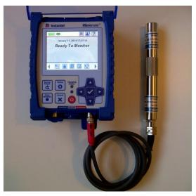
Microphone Connected to the Micromate
