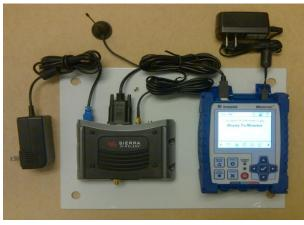
Placement of Modem, Micromate and Cables
