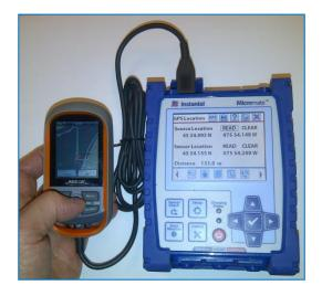
**GPS Connected to Micromate**
