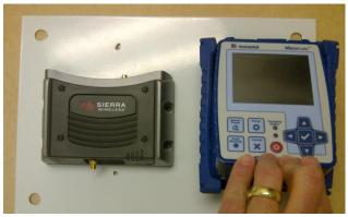
Install the Micromate in the Protective Boot
