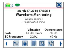
Sample Display for Waveform Monitoring
