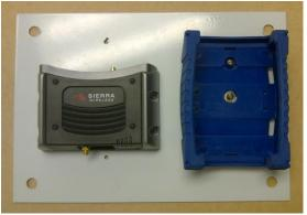
Modem and Protective Boot Secured
