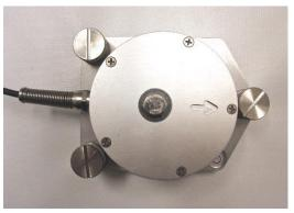
Geophone Mounted with a Leveling Plate
