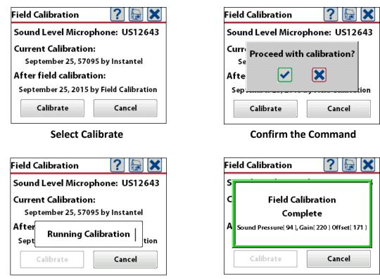
**Micromate Calibrating Sound Level Microphone**
