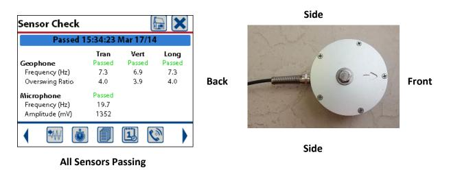
The most common reasons for a failed geophone sensor check are due to the improper leveling or connection of the geophone.
