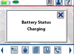
Micromate with External Power Connected
