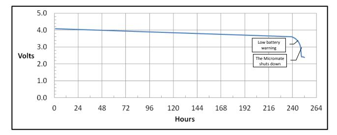
**NOTE:** In this example, elapsed time between the low battery warning and the Micromate shutting down was approximately three hours.
