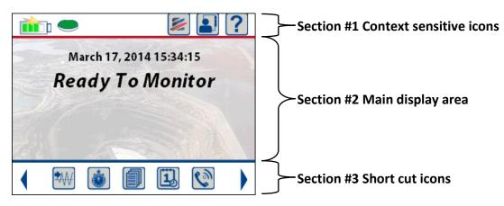
**WARNING: DO NOT** use hard objects, such as pens or hard-tipped styluses to navigate the screen as they may damage the display.
