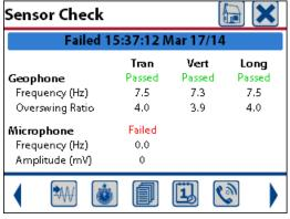
Sensor Check – Microphone Failing
