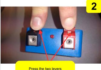
Press the two levers terminals to be able to connect the shooting line.
