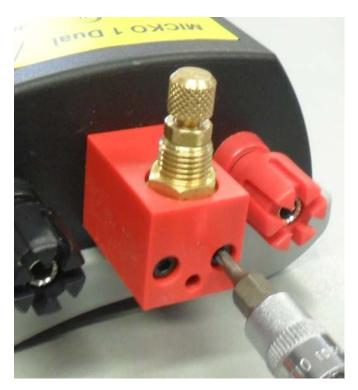
The springs on the back automatically release the block. Make sure that the new block springs have good electric contact, or the spark won't take place. Take a brand new block and place it paying attention to insert the screws and the springs in the correct holes. Screw (rotate clockwise) to settle the new block.
